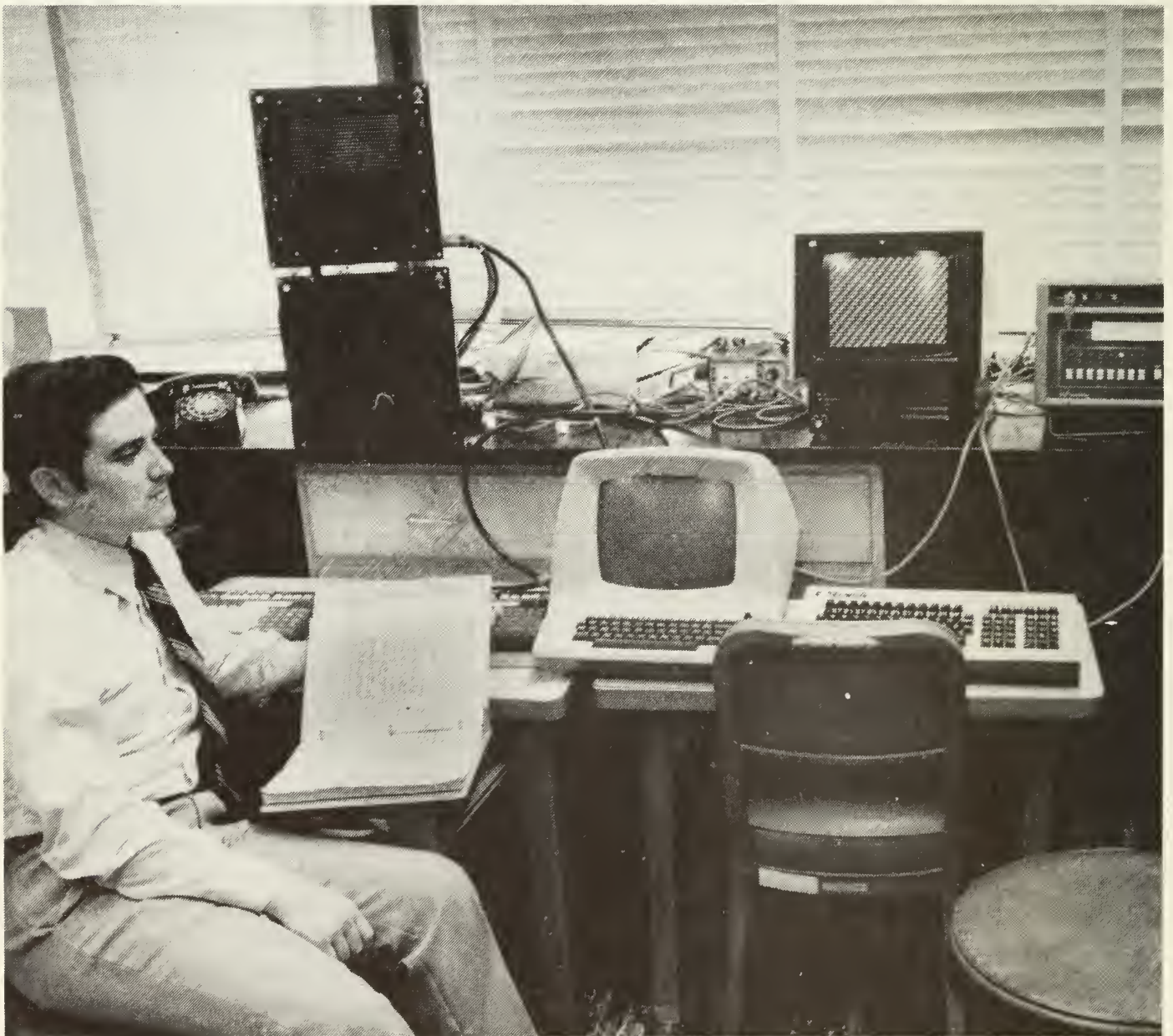
Set-up for shipboard tactical position display that uses a microcomputer driven plasma display
